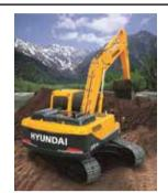
Robex R220-9S with operating weight 21.9 ton now comes with Hyundai Cummins Engine which is newly produces by applying the advance technology of Cummins and production engineering of Hyundai Heavy Industry, will exhibited by Hyundai Machinery Indonesia.
