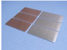
① Active brazing filler material/copper composite material pressed into circuit shape
